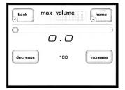
The **max volume** screen allows you to establish a maximum volume setting for your system. This scale runs from 0 to 100, with 100 indicating that you do not want any artificial limit placed on the maximum gain your preamplifier can provide.
